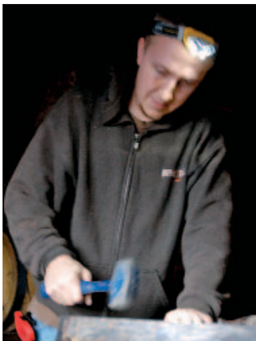
Left to right: plugging the drilled hole after taking a sample; hammering the hoops into place after replacing a barrel head; tools of the trade.
