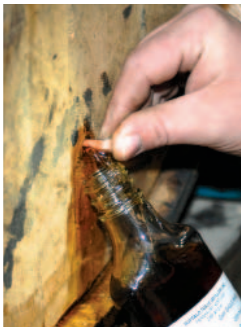
Left to right: plugging the drilled hole after taking a sample; hammering the hoops into place after replacing a barrel head; tools of the trade.
